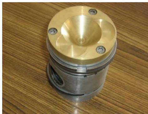
Figure1: An air-gap insulated piston with brass insert
