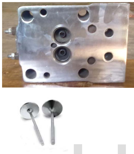
Figure 2: PSZ coated cylinder head and valves
