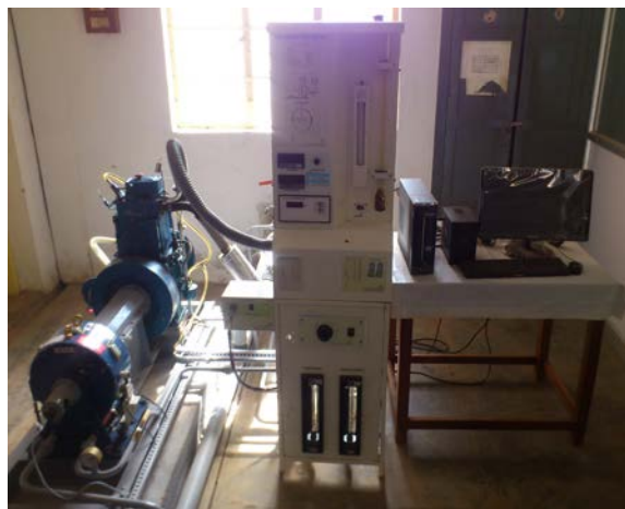
Figure. 3. Experimental set up of Insulated Engine
